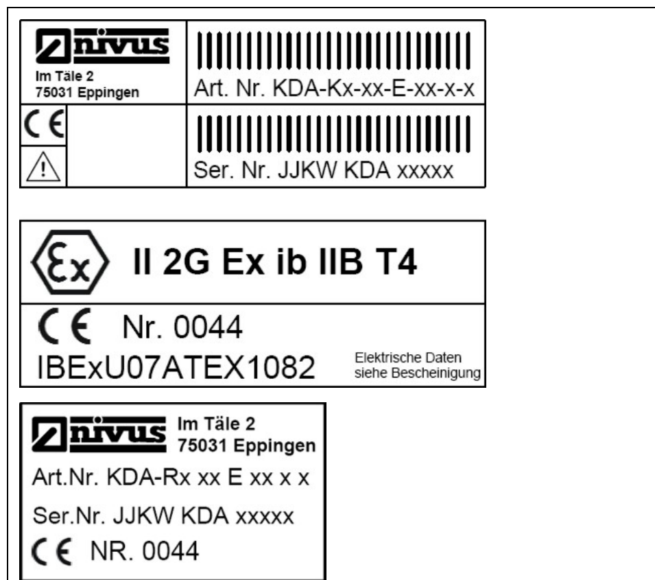
Fig. 3-1 Nameplate flow velocity sensor wedge and pipe
