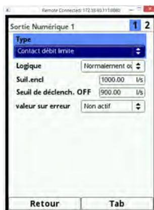
**Fig. 24-8 Programmation contact limite**
