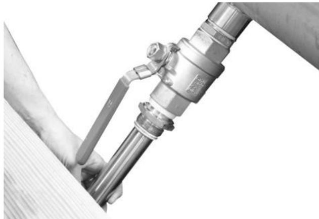
6. Tighten the spigot nut only by hand.
