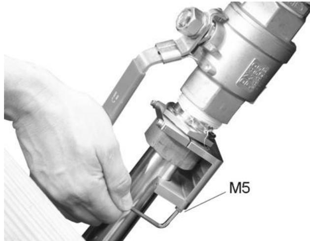
3. Use both M5 hexagon socket screws (see *Fig. 5-28*, Pos. 8) to screw the lower rear clamp element (Pos. 7) to the upper rear clamp element (Pos. 2).
