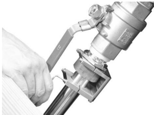
4. Check the tightness of the entire screw joint.
