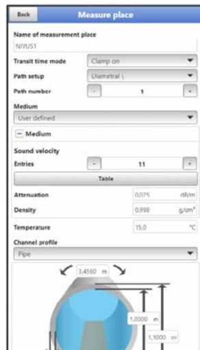
Fig. 42-3 Selection measurement medium
