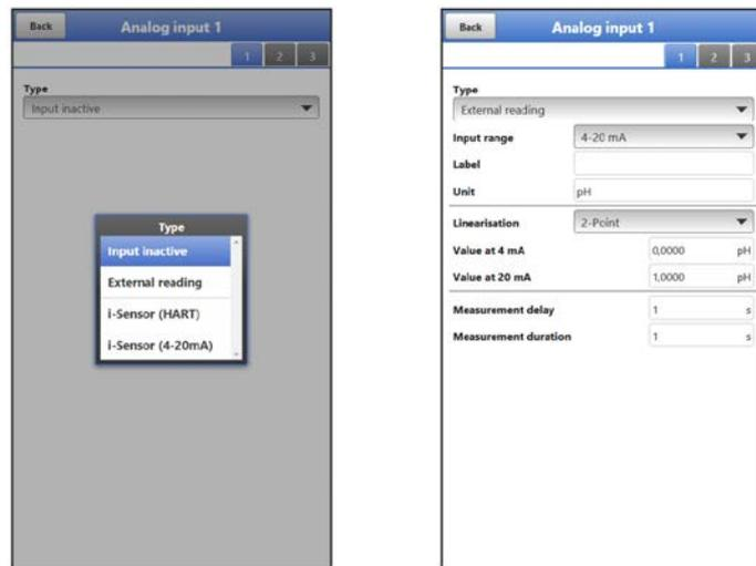
**Fig. 42-9 Analogue input inactive / external measurement value**
