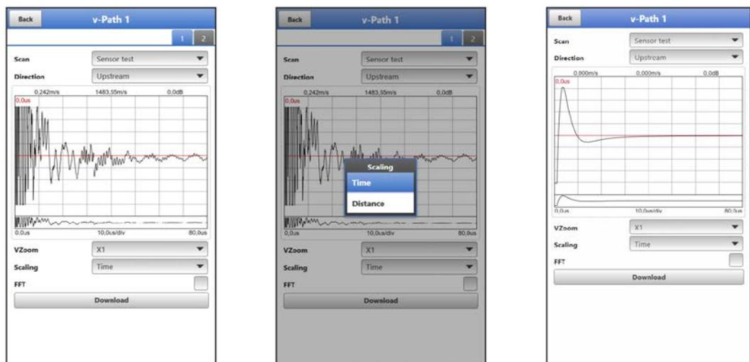
**Fig. 53-6 Signal Analysis Sensor Test / Scaling / No Sensor detected**
