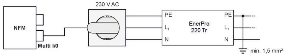
Fig. 26-3 Overvoltage protection for power supply AC general
