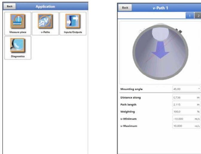
**Fig. 24-1 Output of installation data**
