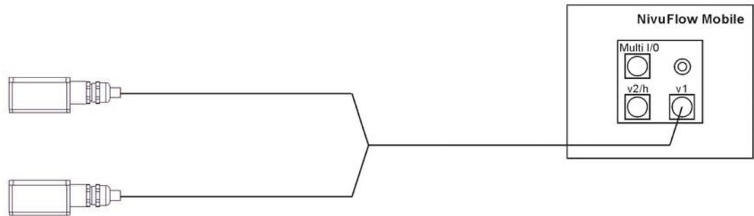
Fig. 26-1 Connection of flow velocity sensors, 1 pair/path
