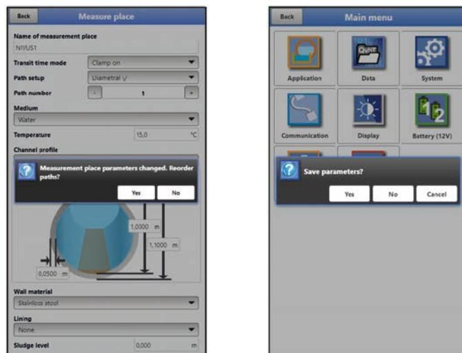
Fig. 33-3 "Realign Paths" and "Save Parameters"
