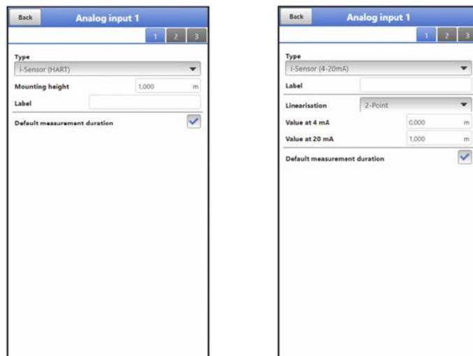
**Fig. 42-10 Analogue input i-Sensor (HART) / i-Sensor (4-20 mA)**
