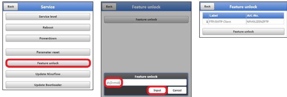
**Fig. 44-10 Activation of the licence in the NFM display tool**
