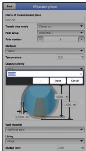
**Fig. 34-2 Entering the pipe data**
