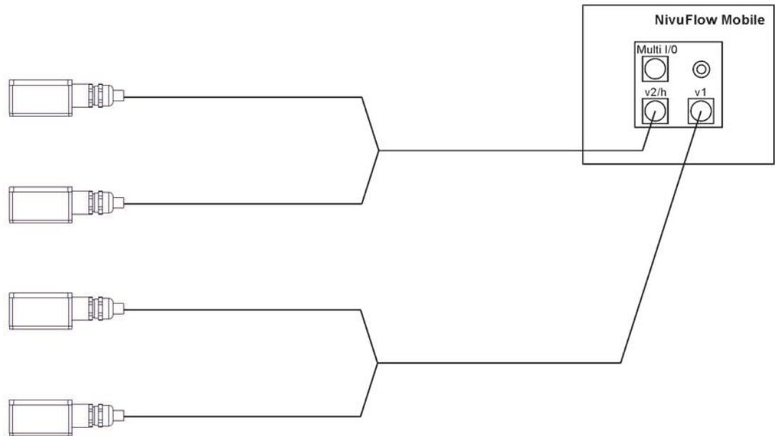
Fig. 26-2 Connection of flow velocity sensors, 2 pairs/paths
