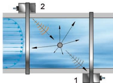
Fig. 20-1 Signal attenuation due to disturbing particles
