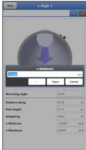
Fig. 42-7 Limiting the Velocity Evaluation
