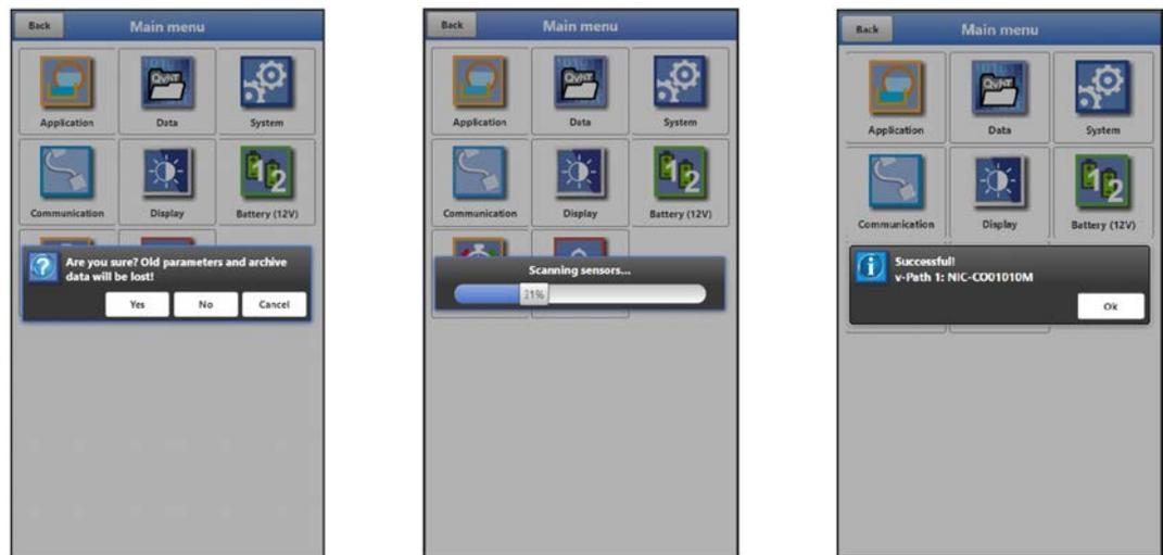
**Fig. 40-2 Security query "Deleting Parameters and Data"**
