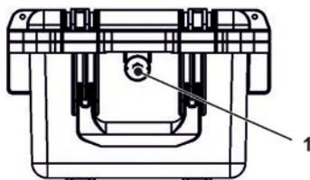
**Fig. 31-1 LED on the front of the NFM**
