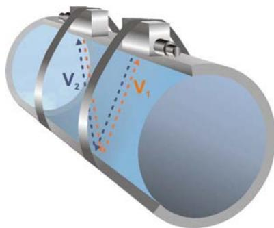
**Fig. 42-2 1-Path measurement, path arrangement: "Diametral V"**
