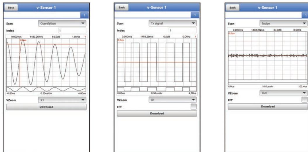
**Fig. 39-2 Signal Analysis Correlation / Tx (Transmission) Signal / Noise**
