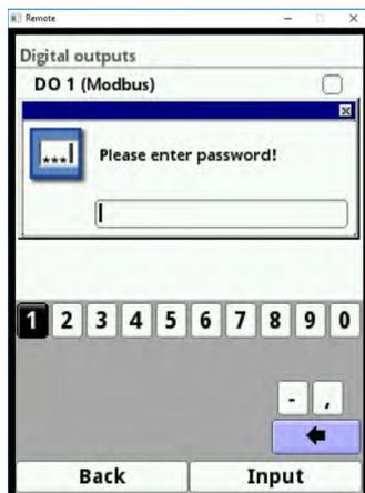
Fig. 33-7 Password-protected simulation
