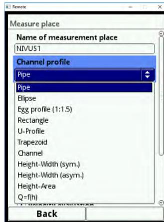
**Fig. 23-2** Selectable channel profiles
