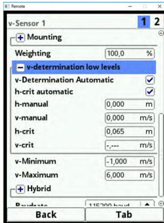
Fig. 23-28 Submenu: v-determination low levels
