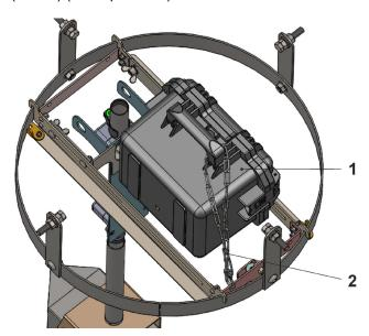
19. Hang the NivuFlow Mobile transmitter by the handle on the hook (Pos. 1) in the inner frame.
