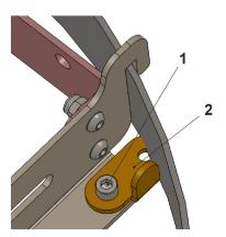
18. Secure the NivuFlow Mobile transmitter (Pos. 1) to the inner frame with a chain (Pos. 2) (holes provided).
