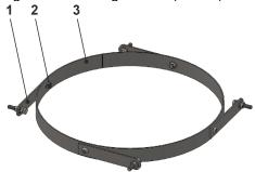
2. Insert the retaining ring into the manhole and hook the suspension plates (Pos. 2) into the (existing) recesses (Pos. 1) on the manhole.
